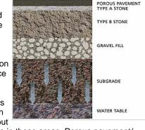
are not impossible to use in these areas. Porous pavement/ pavers should be avoided where activities generate highly contaminated runoff. Areas of low soil permeability, seasonal high groundwater tables (unless overcome by a subsurface tile), and areas close to drinking water supply wells should also be avoided.
